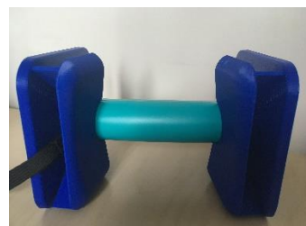
GripAble sitting in two StAbles to place the device horizontal with finger plate facing away
