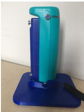
GripAble sitting in the StAble in the vertical position.
