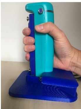
GripAble sitting in the StAble with hand rested on resting plate
